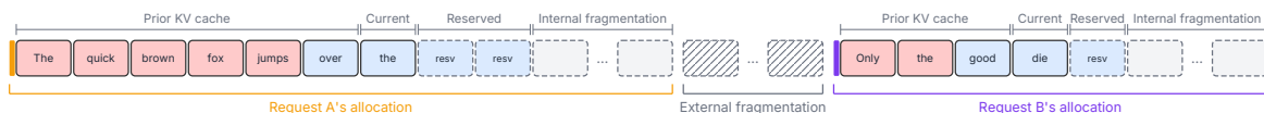
Figure 6.3.: Memory waste with contiguous KV cache allocation. Each request pre-allocates for the maximum sequence length, leaving most of the memory unused.
